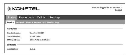
You can find the phone's serial number, network port address and current software version on the **Basic** tab. Settings made by the administrator for the network, time server, SIP accounts and media are on other tabs.
